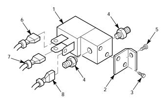
Figure 23 - Fuel Valve Assembly
